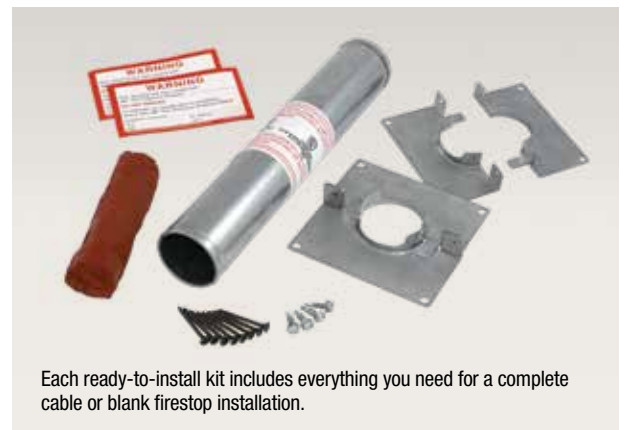
Label holds sleeve together until you need to retrofit around existing cables. Slit label to open sleeve. Close the two halves around the cables.
