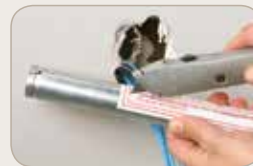
Label holds sleeve together until you need to retrofit around existing cables. Slit label to open sleeve. Close the two halves around the cables.
